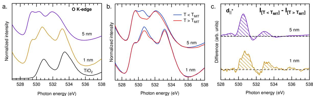
**Figure 7.** (a) O K-edge XAS from two  $\text{VO}_2/\text{TiO}_2$  (100) films with thicknesses of 5 and 1 nm and a  $\text{TiO}_2$  single-crystal reference; (b) O K-edge XAS from the same two  $\text{VO}_2/\text{TiO}_2$  (100) films measured above (red) and below (blue)  $T_{MIT}$ ; (c) intensity difference between high and low temperature O K-edge measurements for the two films.
