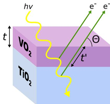
**Figure 1.** A schematic representation of our  $\text{VO}_2$  films of a thickness,  $t$ , grown epitaxially on our  $\text{TiO}_2$  (100) substrates. The photoelectrons, once generated, must travel through some length of the material before they escape the surface and can be detected.
