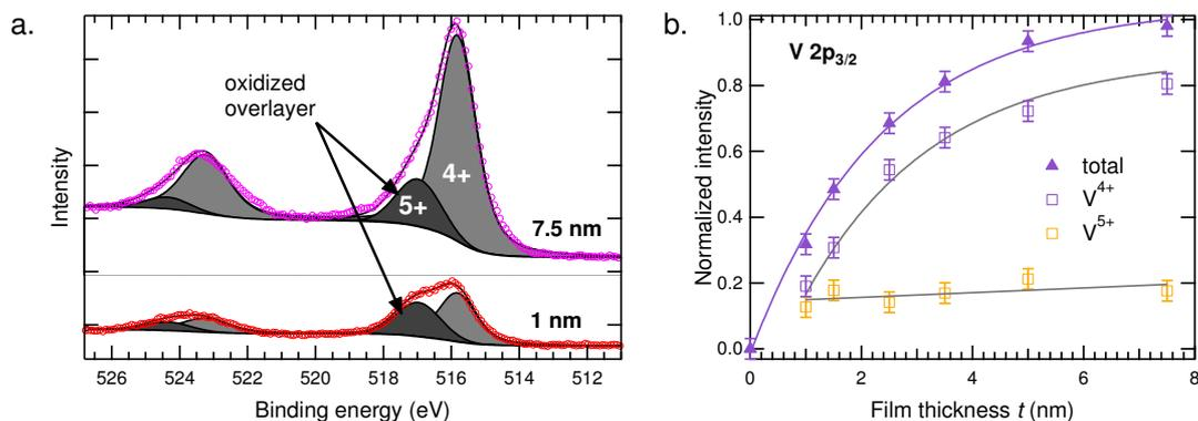
**Figure 3.** (a) HAXPES spectra collected from the 7.5 and 1 nm films. Peak fits show the contributions of  $V^{4+}$  from the film and  $V^{5+}$  from the overlayer; (b) normalized HAXPES signal intensity of the  $V 2p_{3/2}$  showing the  $V^{4+}$  and the  $V^{5+}$  contributions separately *versus* film thickness.
