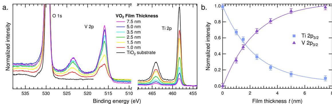
**Figure 2.** (a) X-ray photoelectron spectroscopy (HAXPES) spectra collected from six  $\text{VO}_2/\text{TiO}_2$  (100) thin films with thicknesses varying from 7.5 to 1 nm; (b) normalized HAXPES signal intensity of the  $\text{V } 2p_{3/2}$  and  $\text{Ti } 2p_{3/2}$  versus film thickness.
