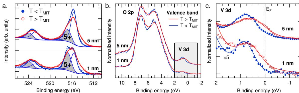
**Figure 6.** (a) V 2p HAXPES measured above (red) and below (blue)  $T_{MIT}$  for two  $\text{VO}_2/\text{TiO}_2$  (100) films with thickness of 5 nm and 1 nm, respectively. Peak fitting results are shown for the low temperature measurement; (b) Valence band HAXPES; and (c) an expanded view of the topmost V 3d states of the same two samples.
