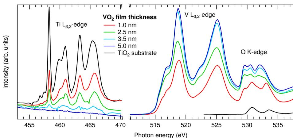
**Figure 5.** Ti  $L_{3,2}$ -, V  $L_{3,2}$ - and O K-edge XAS spectra of four VO<sub>2</sub>/TiO<sub>2</sub> (100) films of different thickness and a TiO<sub>2</sub> single crystal for reference.
