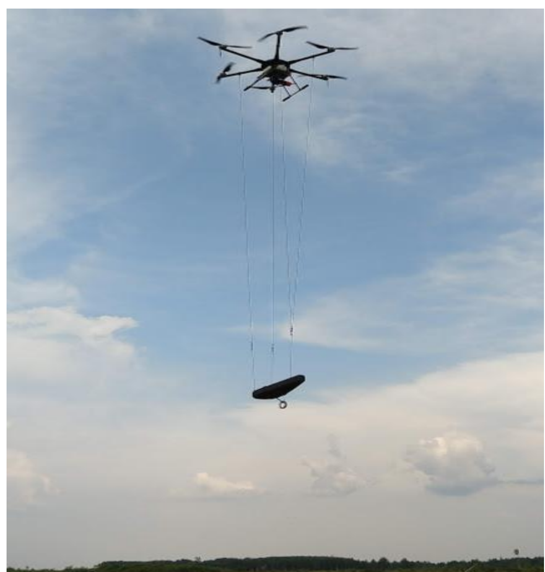
Figure 2: Cicada drone flying the UMT MFAM MagPike over a test-site in Ukraine
