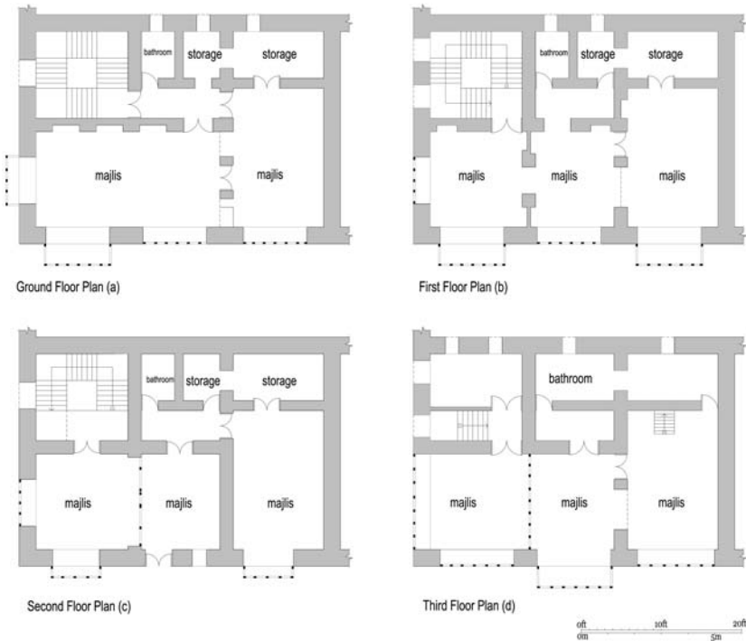
Figure 7. Plans of the bottom four floors of a five-story house in Jidda, Saudi Arabia. Drafted by Anwar Ibrahim, adapted from Bonnenfant, “La maison dans la péninsule arabique,” 775–776.
