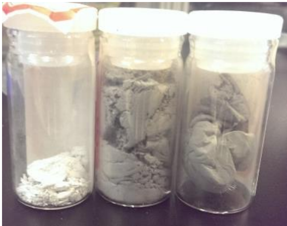
Figure 5-7: Electrospun PMMA doped with 3, 6, and 9 wt% graphene NPs (from left to right).
