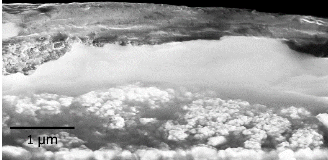
Figure 2-11: Cross-section SEM image of solar cell using PEDOT:PSS as a HTL.
