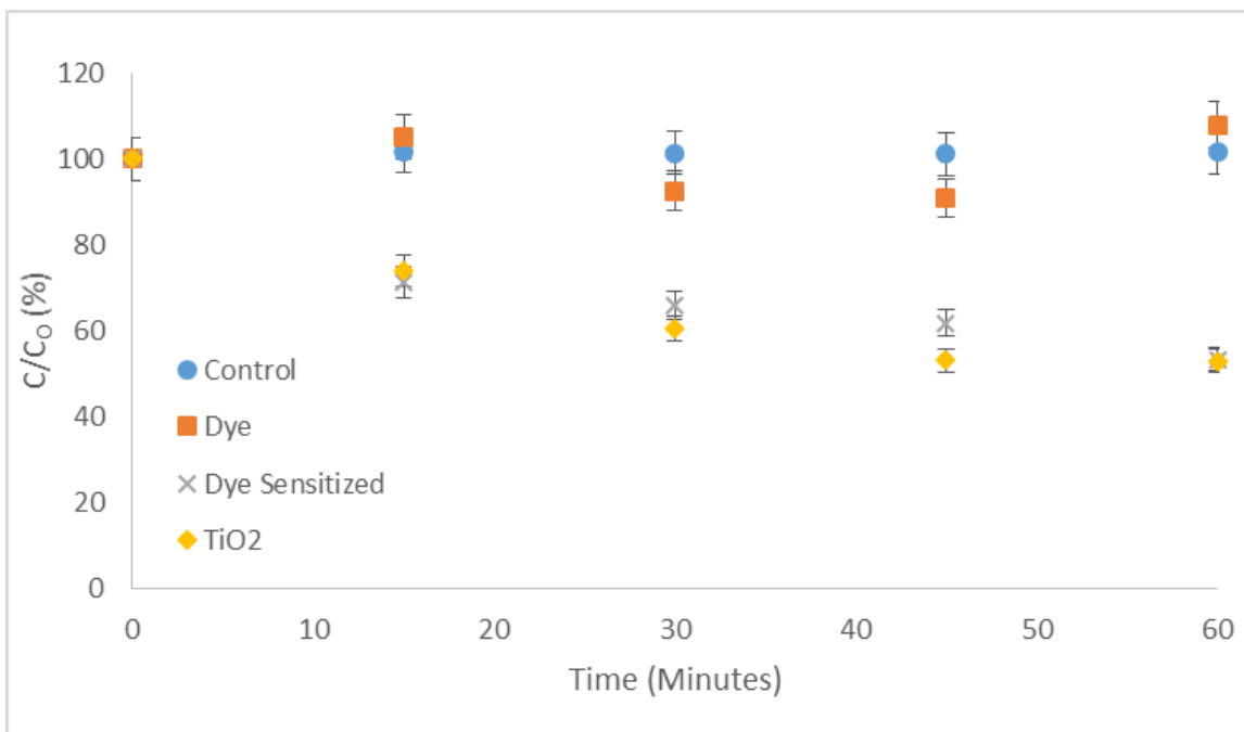
Figure 4-9: Absorption of PAP over time when exposed to no catalyst, \text{Ru}(\text{dcbpyH}_2)_2\text{Cl}_2 , \text{TiO}_2 fibers and \text{Ru}(\text{dcbpyH}_2)_2\text{Cl}_2 - sensitized \text{TiO}_2 fibers in dark and under visible irradiation.
