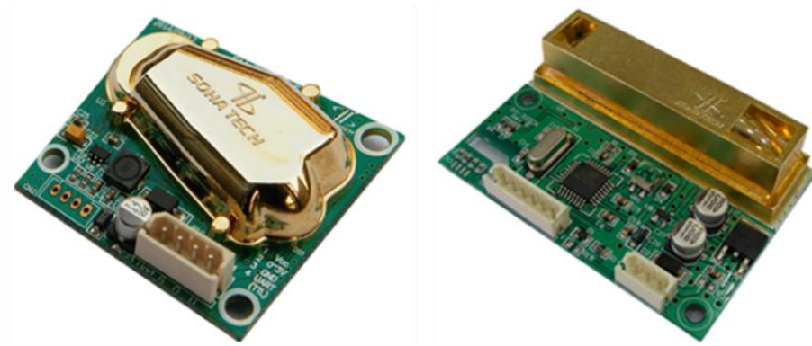
Figure 1.6: Commercially available CO2 Sensor which uses lid as gas cavity
