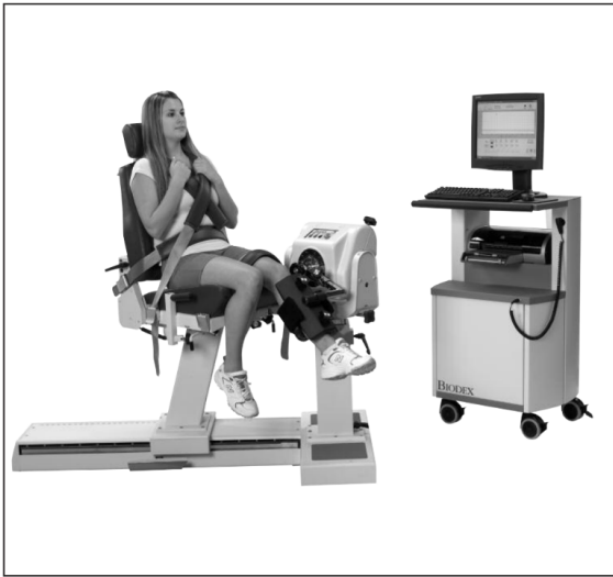
Figure 2. Biodex knee flexion/extension setup. Individuals were seated and strapped to the equipment as pictured above. The two buckles going across the chest were not placed across the individual. The lateral epicondyle of the knee was lined up with the dynamometer
