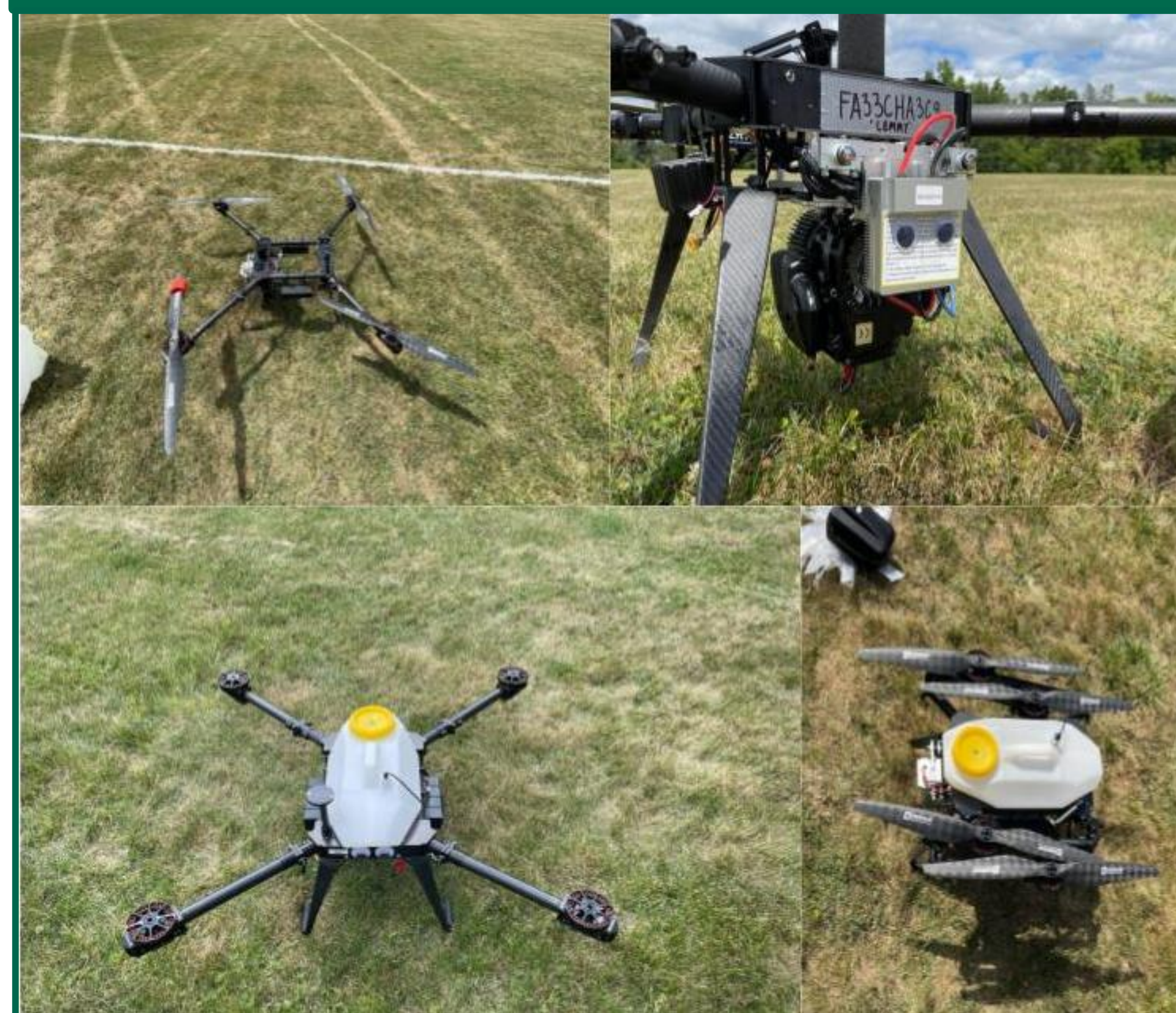
Image Set 2: The FOXTECH Thea 140 pro hybrid UAV, nicknamed 'Lemmy' The large plastic object in the middle is the fuel tank, The top right picture shows the generator off
