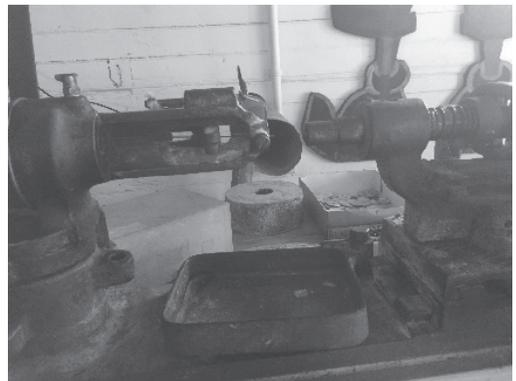
Figure 4. Finishing machine used to drill eyes. (Photo by Siara L. Biuk, 2016.)
