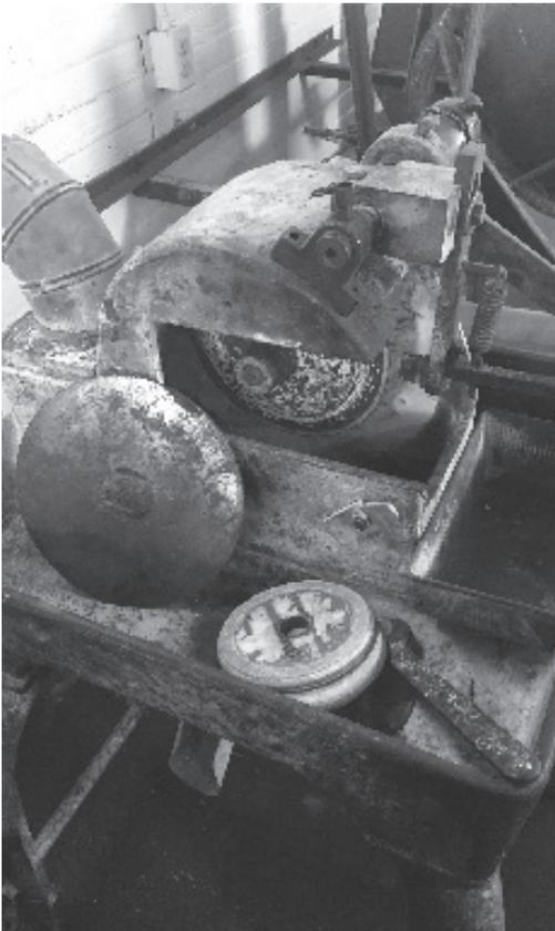
Figure 3. Machine used to slice blanks to even thickness. (Photo by Siara L. Biuk, 2016.)
