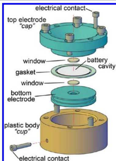
**Figure 7.** Schematic of AMPIX electrochemical cell.<sup>39</sup> Reproduced with permission from ref 39. Copyright 2012 International Union of Crystallography.
