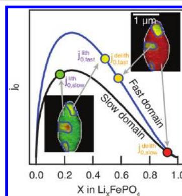
**Figure 11.** Relationship between measured exchange current density and degree of (de)lithiation. Because the skewed  $j_0$  peaks at  $x \approx 0.25$ , the value of  $j_0$  for the fast domains is several times that of  $j_0$  for the slow domains during delithiation, but the two quantities are comparable during lithiation. Reprinted with permission from ref 36. Copyright 2016 AAAS.
