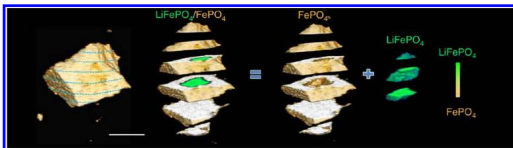
**Figure 12.** Sliced view of  $\text{LiFePO}_4$  at a highly delithiated state. The sliced view reveals 3D internal core–shell phase distribution. Scale bar,  $10\ \mu\text{m}$ . Reprinted from ref 23, licensed under CC-BY 4.0.
