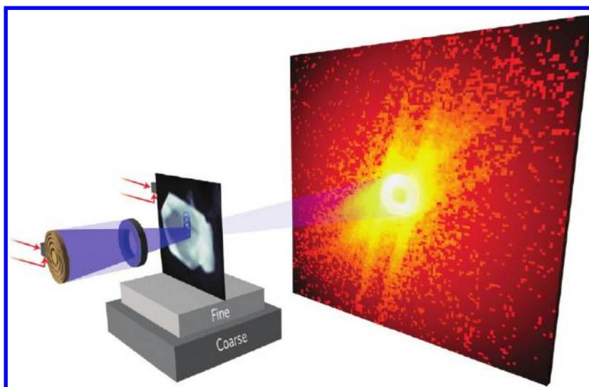
**Figure 6.** Schematic of a soft X-ray ptychographic microscope. An incoming X-ray beam is focused onto the sample by a zone plate and order sorting aperture. The coherent diffraction pattern is collected by a CCD.<sup>10</sup> Copyright 2014 John Wiley and Sons. Reprinted with permission from ref 10. Copyright 2014 Macmillan Publishers Limited.
