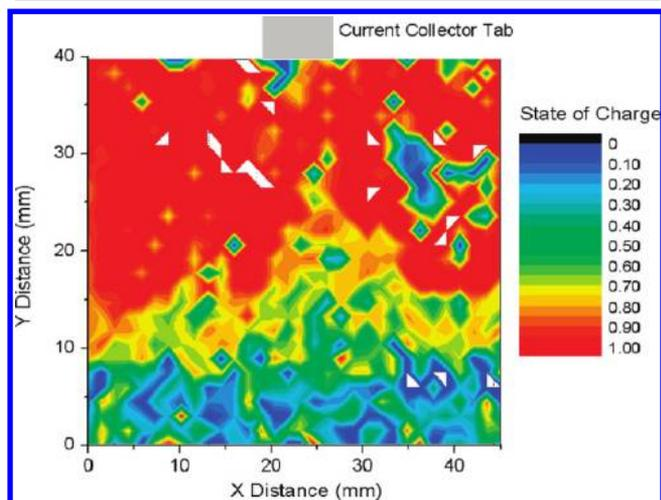
**Figure 13.**  $\text{FePO}_4$  phase concentration profile of the prismatic electrode at 50% state-of-charge. Reprinted with permission from ref 57.
