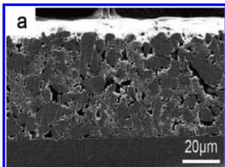
**Figure 2.** Scanning electron microscope image of the cross-section of a typical battery electrode. Multiple individual particles can be seen that participate in the electrochemical reaction. Reprinted from J. Choi et al. Improved high-temperature performance of lithium-ion batteries through use of a thermally stable copolyimide-based cathode binder. *J. Power Sources* **2014**, *252*, 138–143, with permission. Copyright 2014 Elsevier.
