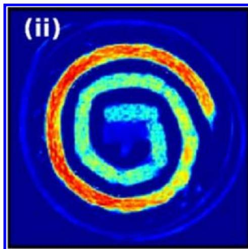
**Figure 14.** Data collected for cycled Ni-MH cell showing intensity at  $q = 1.36\ \text{\AA}^{-1}$ , representing the cathode phase.<sup>58</sup> Copyright 2015 The Authors. Published by ECS. Creative Commons Attribution 4.0 License (CC-BY). Full text: <http://jes.ecsdl.org/content/162/7/A1310.full>.
