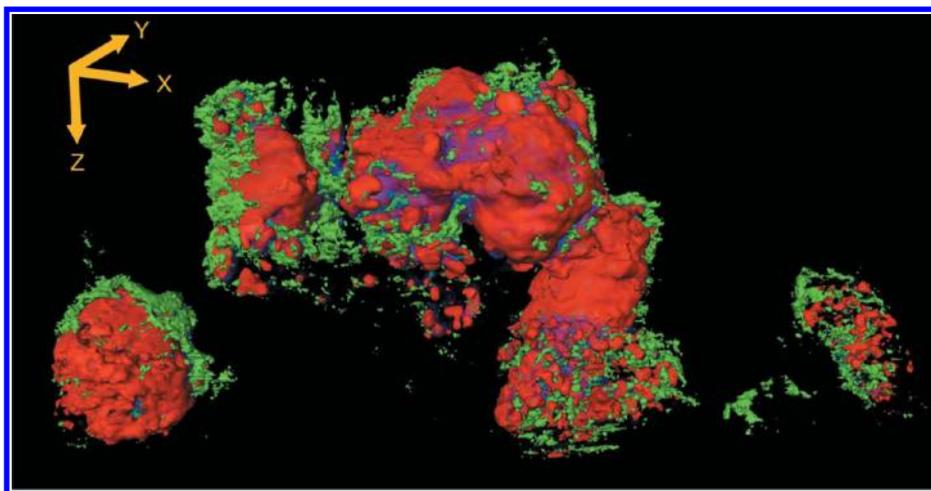
**Figure 9.** Reconstructed three-dimensional XANES tomography perspective rendering of three-dimensional data set of NiO cathode.<sup>18</sup> Reproduced with permission from ref 18. Copyright 2011 International Union of Crystallography.
