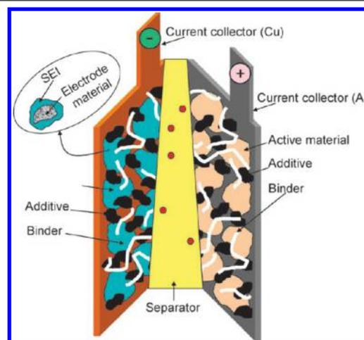
**Figure 1.** Schematic of a typical battery. The electrodes are made of multiple individual particles that participate in the electrochemical reaction (denoted as “active material”). Reproduced from ref 5 with permission. Copyright 2009 the Royal Society of Chemistry.
