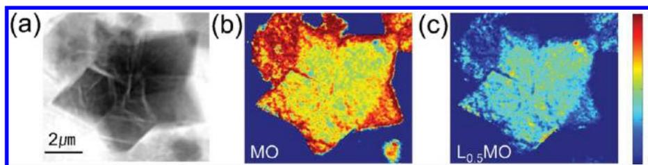
**Figure 10.** Preferential growth of  $\text{Mn}_2\text{O}_4$  along cracks at 4.09 V. (a) Inverted optical density image collected at 6700 eV. Heat maps where color contrast scales with the ratio of spectral standards of (b)  $\text{Mn}_2\text{O}_4$  and (c)  $\text{Li}_{0.5}\text{Mn}_2\text{O}_4$  in each pixel. Reprinted with permission from ref 53. Copyright 2014 John Wiley and Sons.
