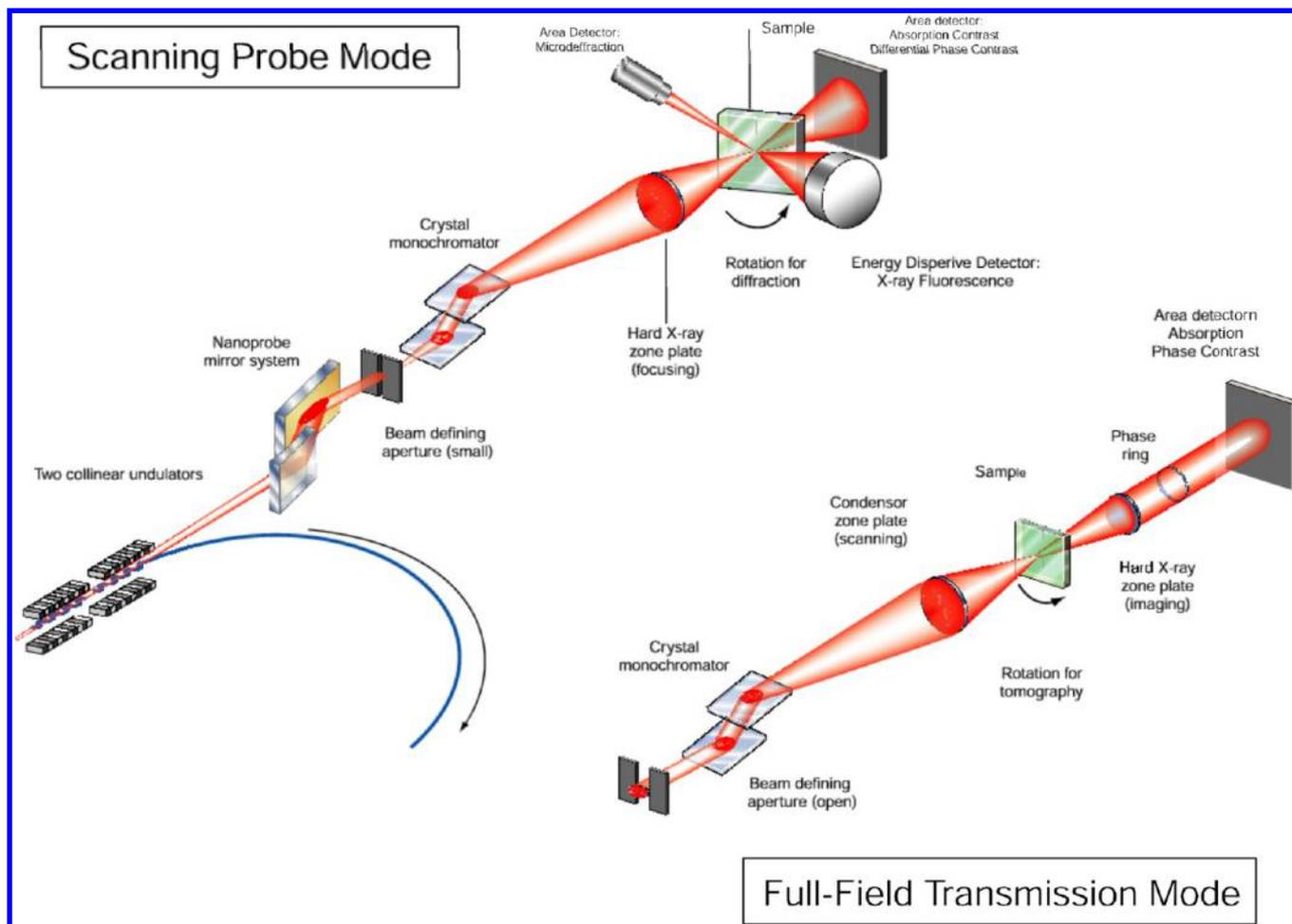
**Figure 4.** Illustration of experimental configurations for (a) scanning probe and (b) full-field imaging synchrotron hard X-ray microscopy methods. Reprinted with permission from Maser et al. Development of a Hard X-ray Nanoprobe Beamline at the Advanced Photon Source. *Microsc. Microanal.* 2005, 11, 680–681. Copyright 2005 Cambridge University Press.
