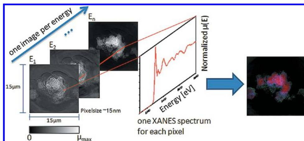
**Figure 5.** Reduction of TXM stacks to form chemical maps. A full spectrum is extracted for each pixel and used to calculate the chemical state of the material and then converted to a color.<sup>18</sup> Reproduced with permission from ref 18. Copyright 2011 International Union of Crystallography.
