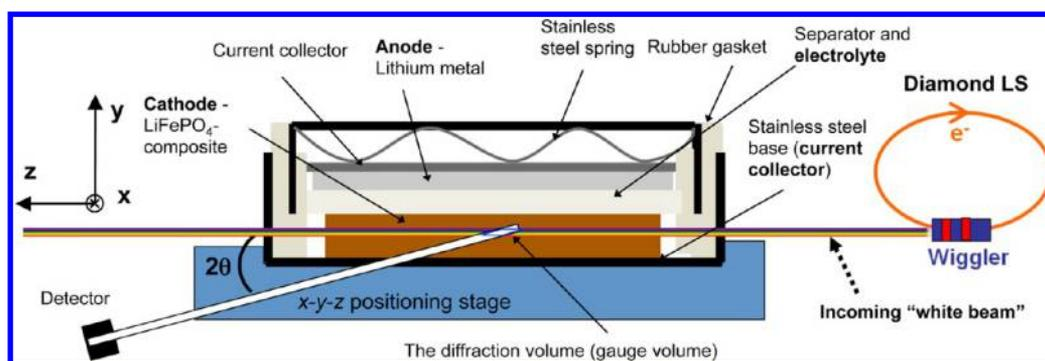
**Figure 15.** In situ EDXRD setup at the Diamond Light Source and the cross section of a coin-cell battery placed on an  $x$ - $y$ - $z$  position stage. X-rays penetrate the stainless steel casing and the diffracted X-rays are detected at a fixed angle. Reprinted with permission from ref 32.
