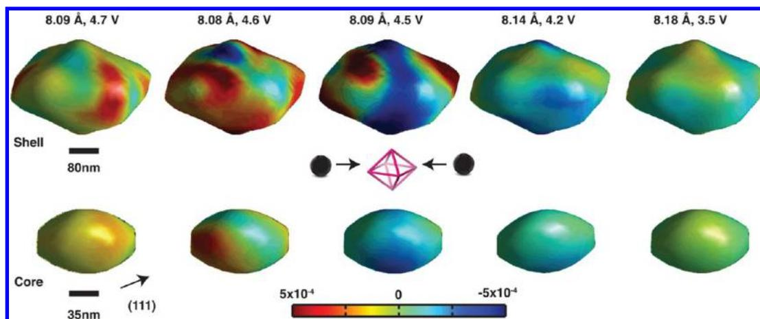
**Figure 16.** Isosurface projections of strain evolution in  $\text{LiNi}_{0.5}\text{Mn}_{1.5}\text{O}_4$  nanoparticle. The shell and core both show inhomogeneous strain during discharge. Images are labeled by their respective lattice constant values and open circuit voltages. The highest lattice strain occurs immediately prior to the phase transformation. Reprinted with permission from ref 63.
